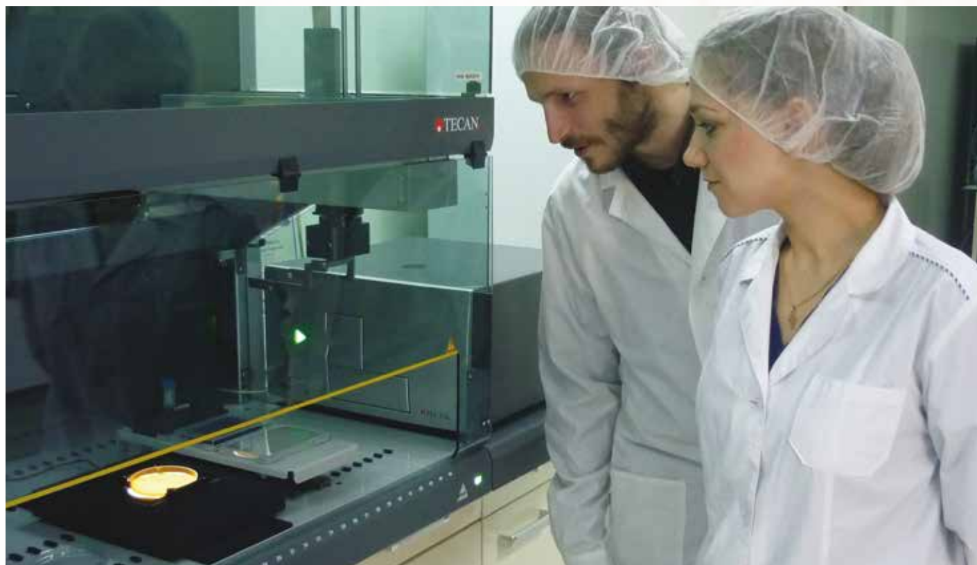
The Pickolo module offers fully automated colony picking, plate seeding and MALDI spotting for Soyuzsnab
