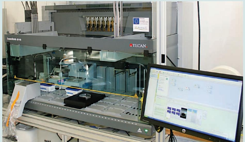
Mejoran developed a unique colony picking procedure on a Freedom EVO with an integrated SciRobotics Pickolo module
