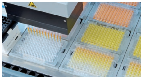
Pipetting with a single row of 12 disposable tips e.g. for serial dilutions.
