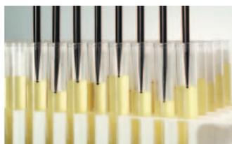
Pressure-based liquid level detection
