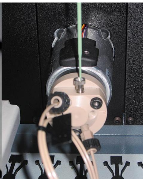
*Direct inject into an integrated GC/HPLC sample loop on a Freedom EVO deck with the liquid handling arm.*
