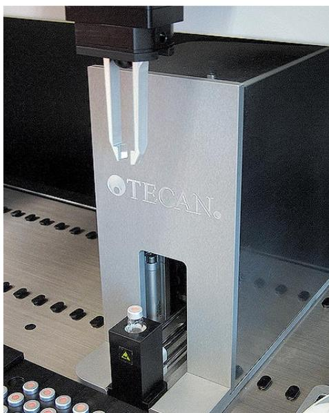
*An integrated vial crimping station with automated tube handling arm.*
