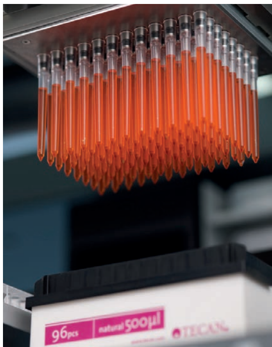
500 µl in the 96-well format with the EVA (Extended Volume Adapter) plate.
