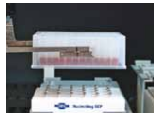
Magnetic extraction – 96-well magnetic separator
