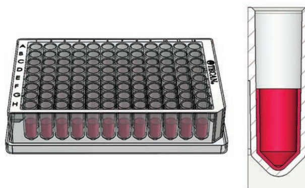
Graphical representation of the Tecan AC Extraction Plate (left) and a cross section of a single well (right), showing the presence of the TICE coating to approximately half the well's height.
