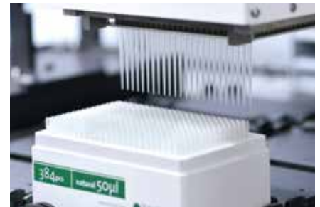
Multiple Channel Arm picking up one row of 24 50 µl tips
