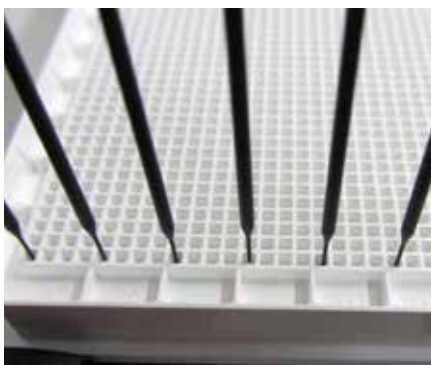
Pipetting into a 1,536-well microplate with the Flexible Channel Arm and Te-PS™ tips
