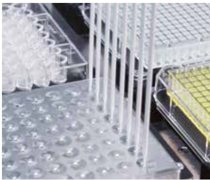
Cap piercing using washable fixed tips with the liquid displacement Flexible Channel Arm
