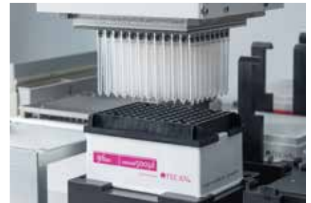
Multiple Channel Arm picking up 96 500 µl disposable tips
