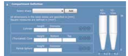
Elegant labware definition enables accurate calculation of detected liquid volumes
